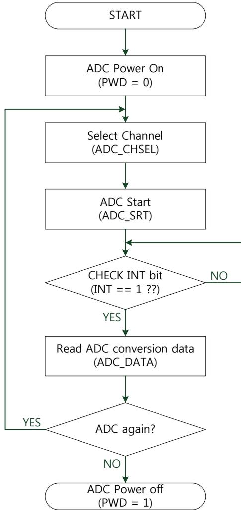
Figure 23. The ADC operation flowchart with non-interrupt
