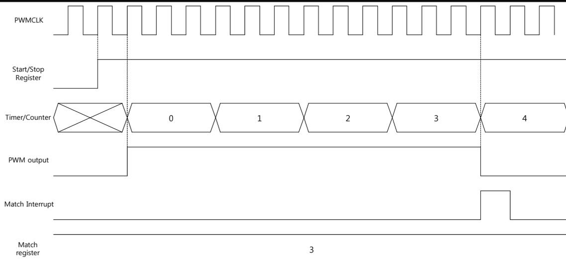
Figure 35 The PWM output up to match register
