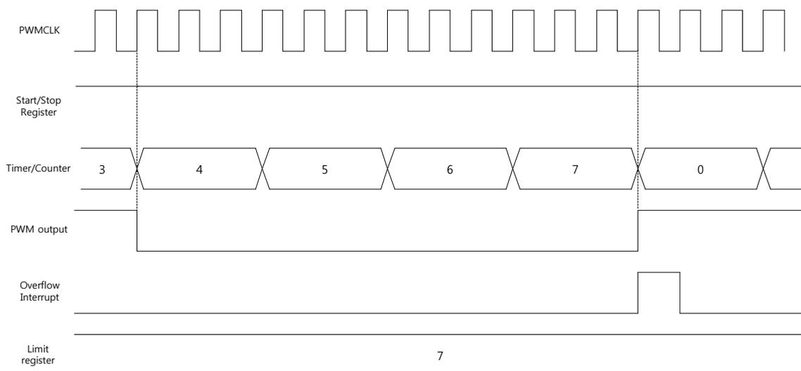
Figure 36 The PWM output up to limit register
