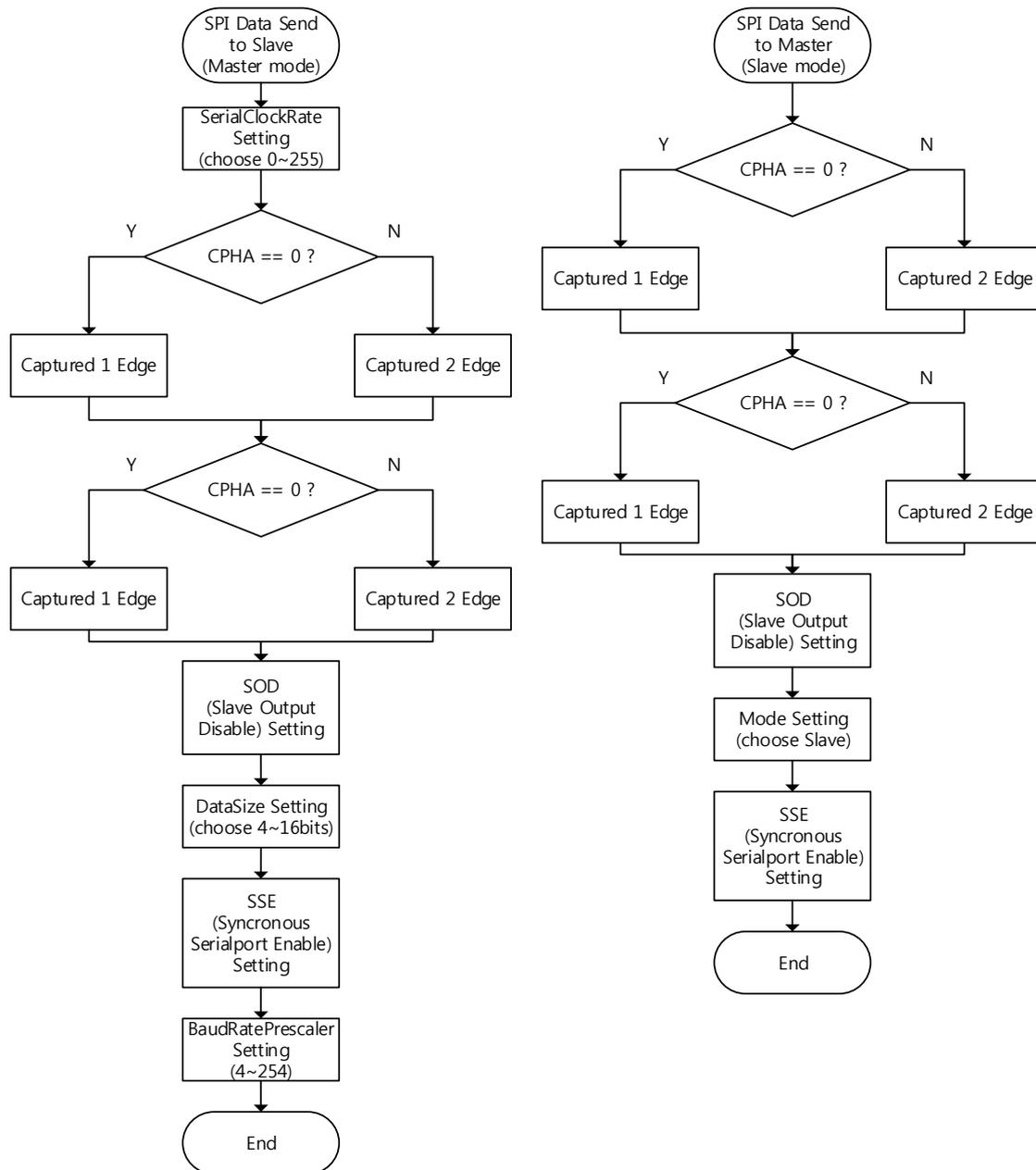
Figure 80. how to setting SPI mode flow chart
