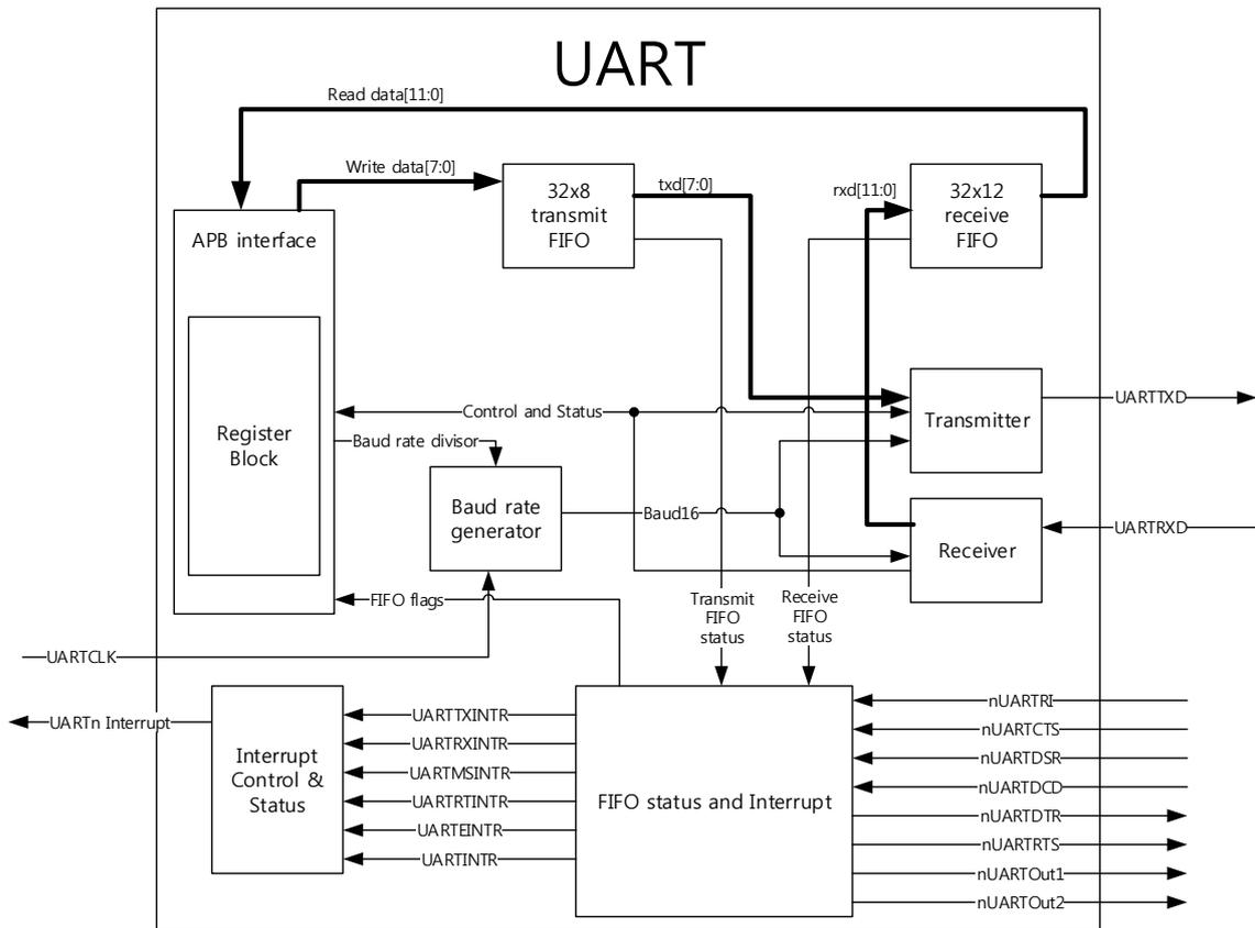
Figure 57. UART0,1 Block diagram
