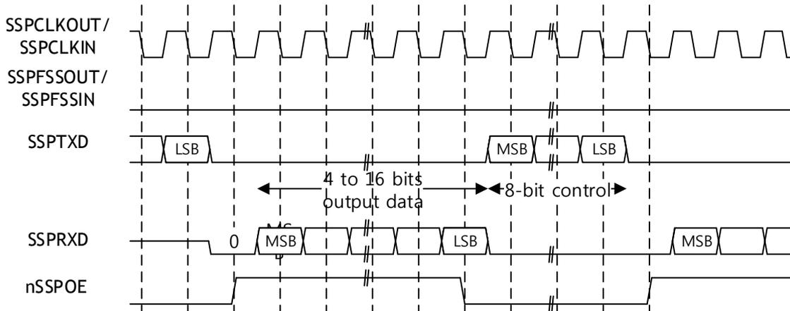
Figure 76. National Semiconductor Microwire frame format, continuous transfers
