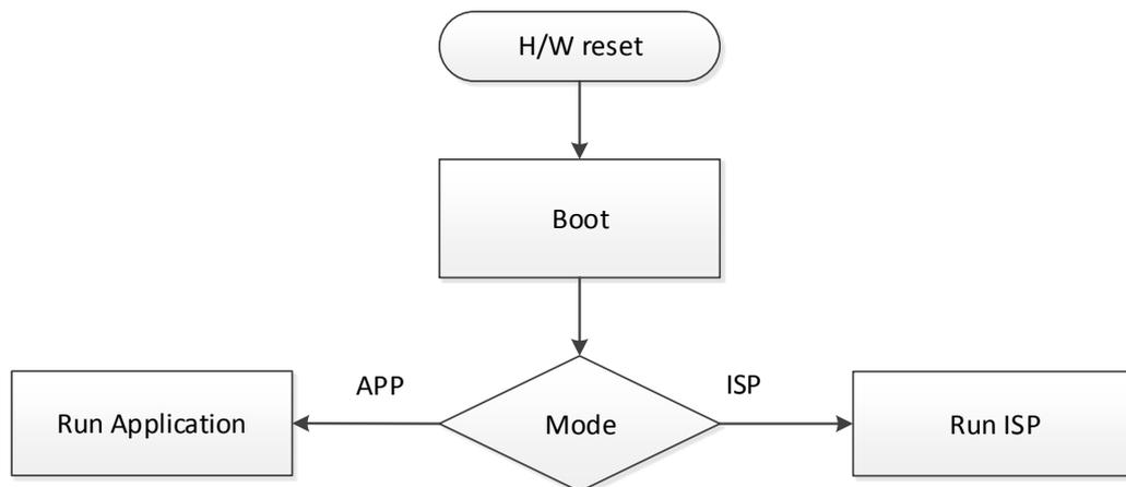
Figure 6. operation of boot code
