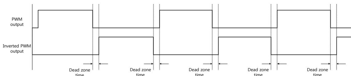
Figure 37 PWM waveform with dead zone time
