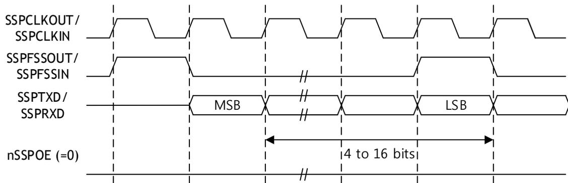
Figure 68. Texas Instruments synchronous serial frame format, continuous transfers
