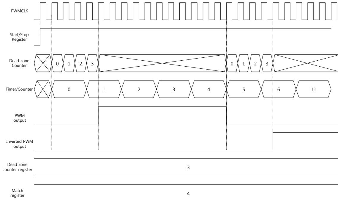
Figure 38 PWM waveform with dead zone counter
