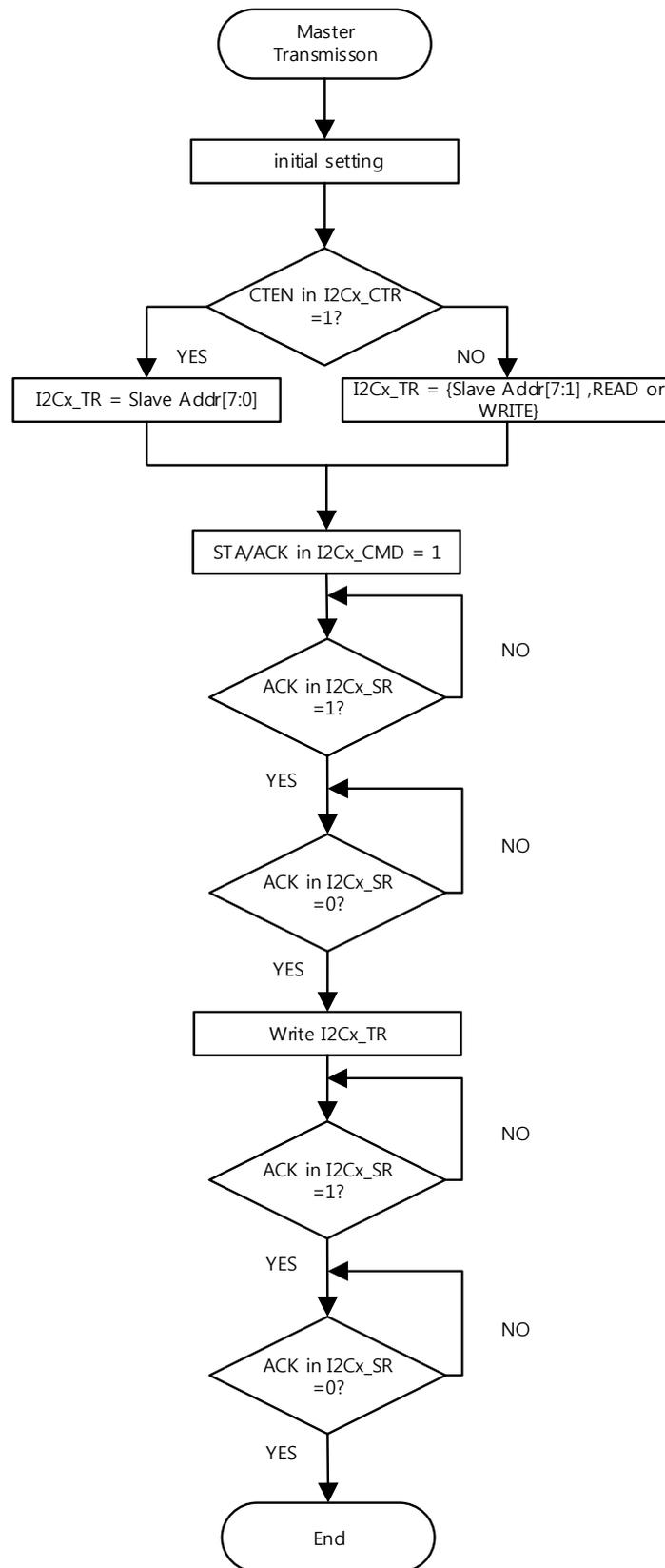
Figure 54. Master TRANSMIT with ADDR10=0 in the I2Cx\_CTR
