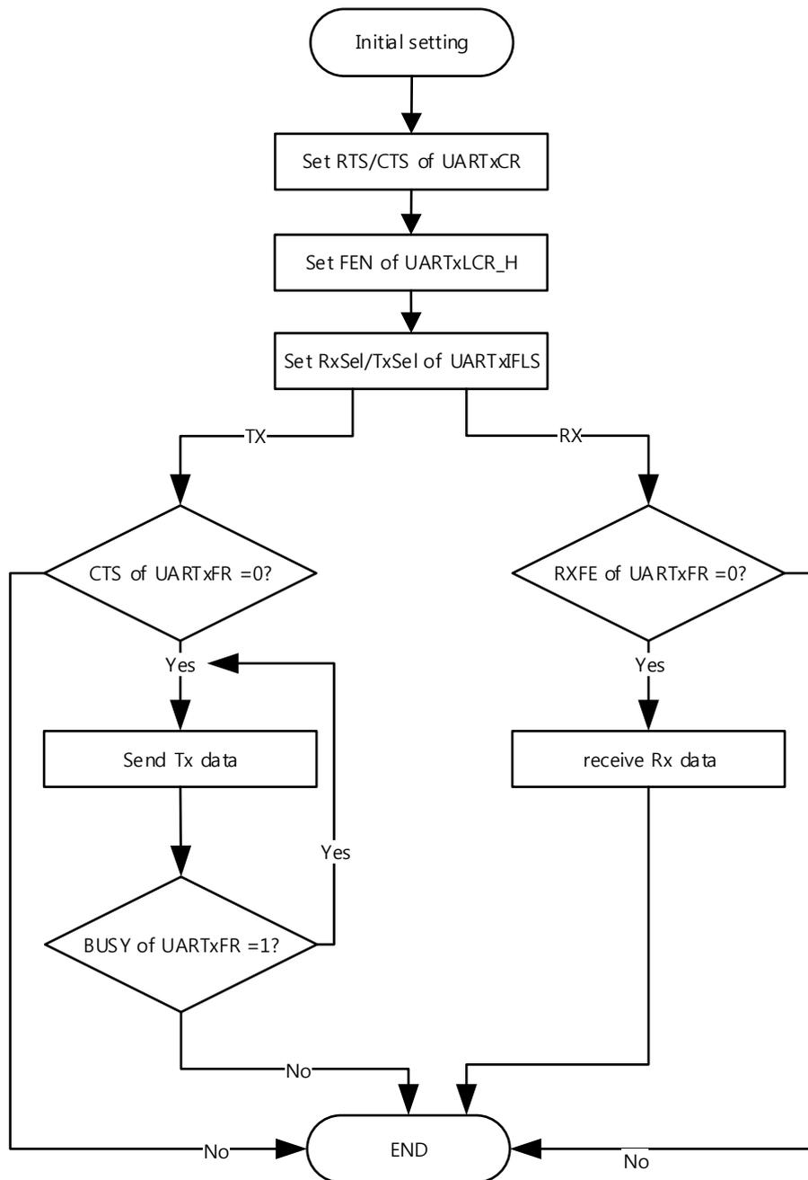
Figure 64. Algorithm for setting CTS/RTS flowchart
