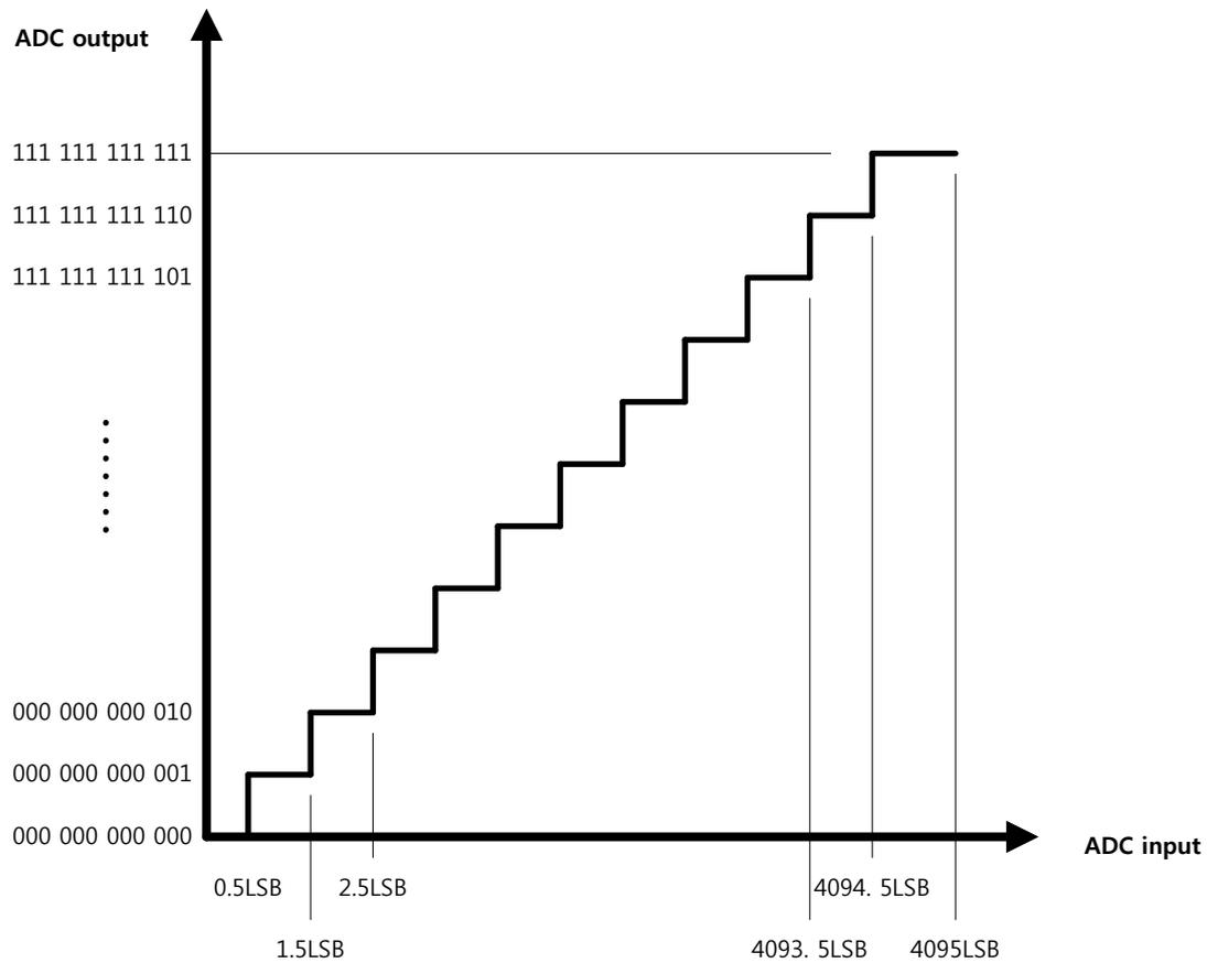
Figure 82. ADC transform function
