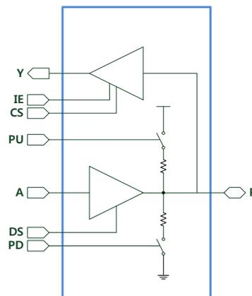
Figure 14. function schematic of digital I/O pad
