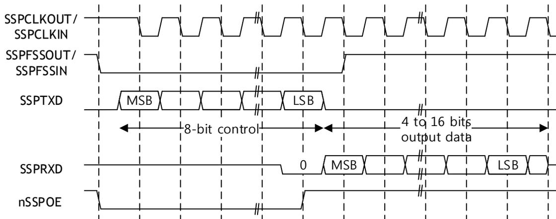
Figure 75. National Semiconductor Microwire frame format, single transfer
