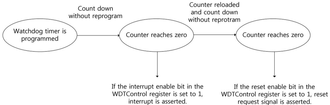
Figure 44 Watchdog timer operation flow diagram
