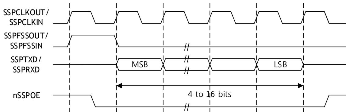
Figure 67. Texas Instruments synchronous serial frame format, single transfer
