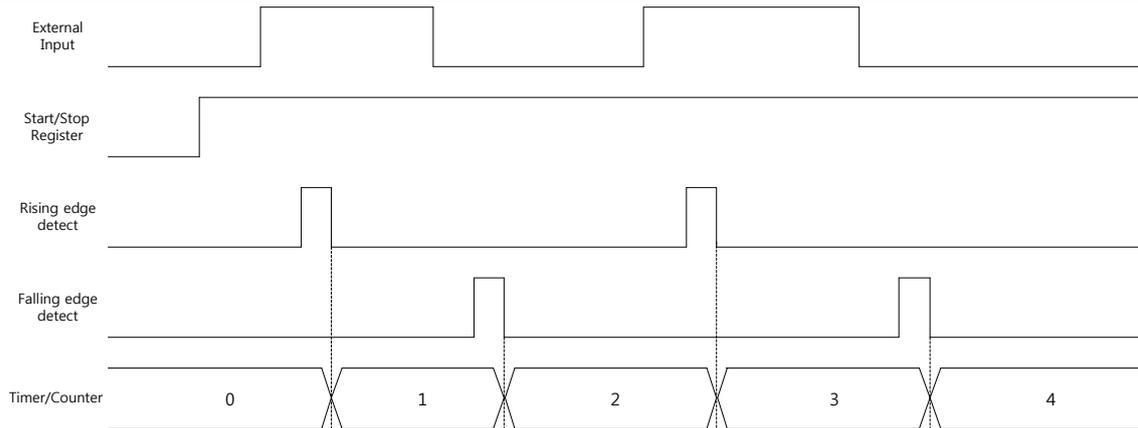
Figure 32 Counter mode with rising and falling edge
