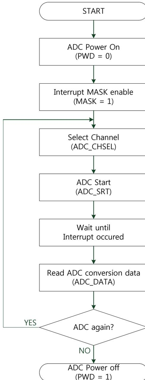
Figure 24. The ADC operation flowchart with interrupt
